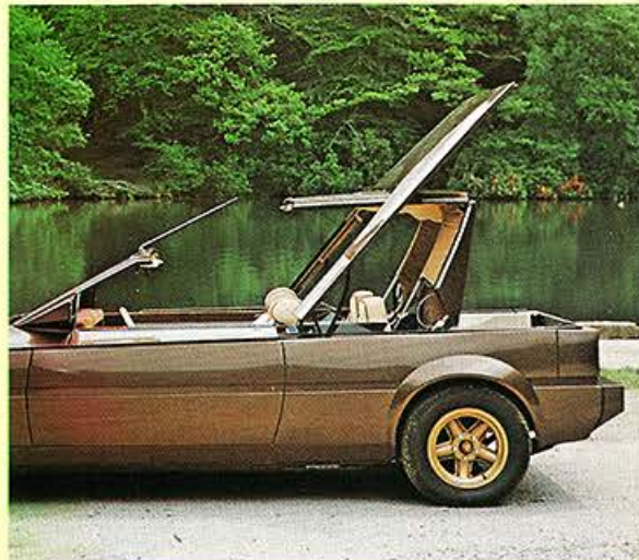
Press a button and the Forté's electro-hydraulic system makes the roof disappear into the boot.
