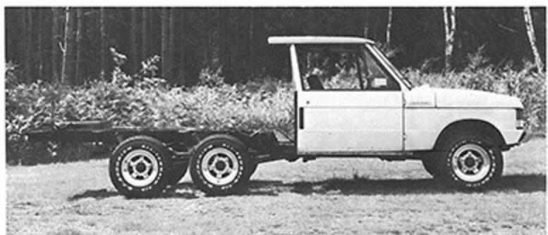
Six wheel Range Rovers are used for both limousines and for a wide variety of military and commercial applications with an up-rated 2.2 tons payload.
