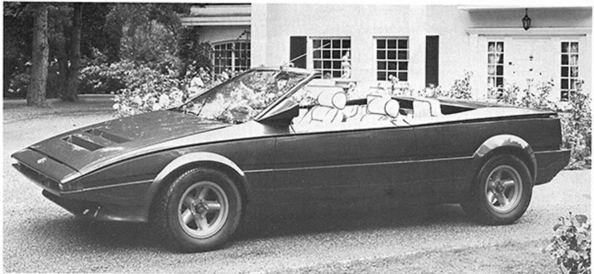
Created by Rapport's own design team, the Forté has been described as the ultimate sports car. It has saloon car comfort due to its patented roof design. At the press of a button, the metal roof automatically folds down into the boot. It also features an electrically operated aerofoil similar to the Ritz. Powered by Jaguar 3.4, 4.2 or 5.4 litre engines. Turbo-charging is optional.
