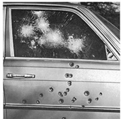
When seen being driven along the road, Rapport Armalite's bullet-resistant cars are indistinguishable from their standard counterparts. The passenger compartment is encased in special materials which are lighter and more efficient than traditional metals. All glass is bullet-resistant; the fuel tank is explosion-proof and many additional security devices can be fitted.
